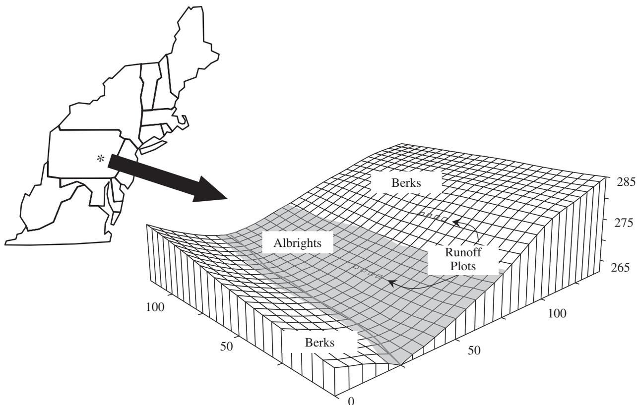
**Fig. 1.** Location of study site in eastern USA and 1-m contour map of hillslope showing location of runoff plots in Albrights (shaded) and Berks (unshaded) soils. Each set of plots includes four abutting pairs of 1 by 2 m runoff plots (eight plots per set).
