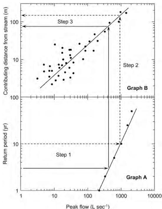
Fig. 3. Nomograph for determining contributing distance as a function of return period for the FD-36 watershed. In Step 1, peak stream flow is determined from the specified return period in graph A (adapted from Flippo, 1977); in Step 2, peak flow from graph A is matched to graph B; and in Step 3, graph B peak flow provides contributing distance from FD-36 data.
