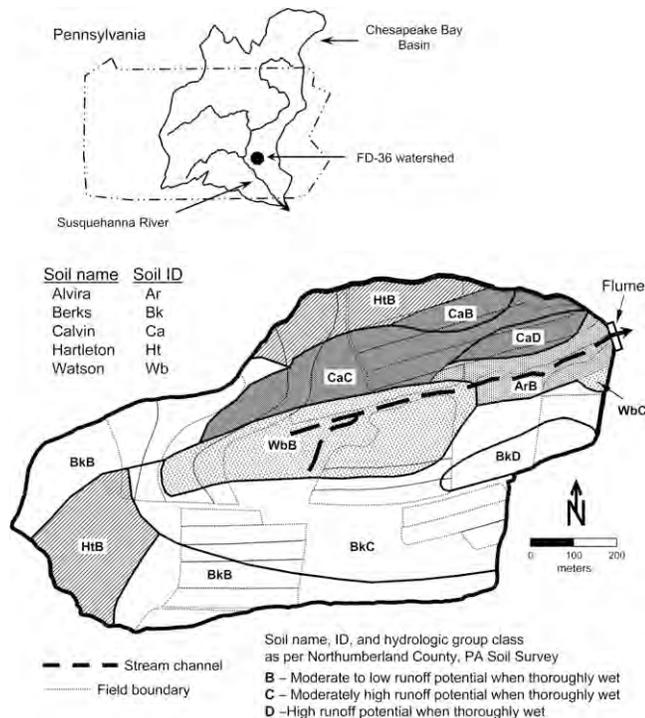
Fig. 1. The FD-36 watershed, soil series and drainage class distribution, field boundaries, and location within Pennsylvania and the Chesapeake Bay Watershed (USDA-NRCS, 1993).
