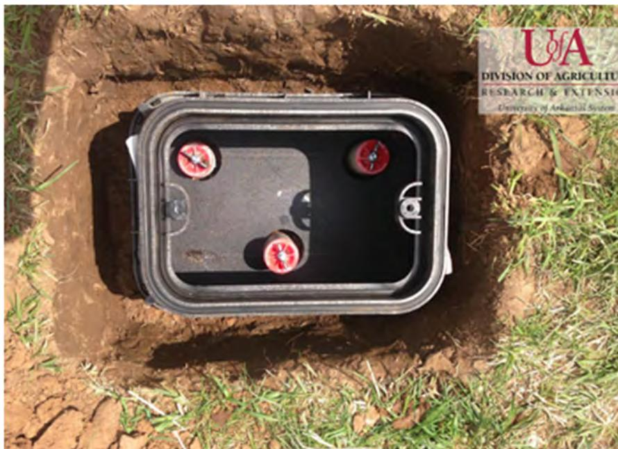
Figure 4. Construction of belowground piezometer.
